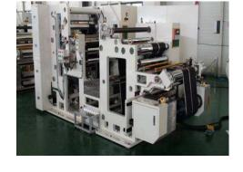
Aqueous based anode coating process (Titanate material)
