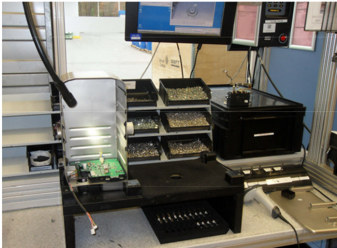
Pre-Assembly Housing with BMC (Pick to Light)
